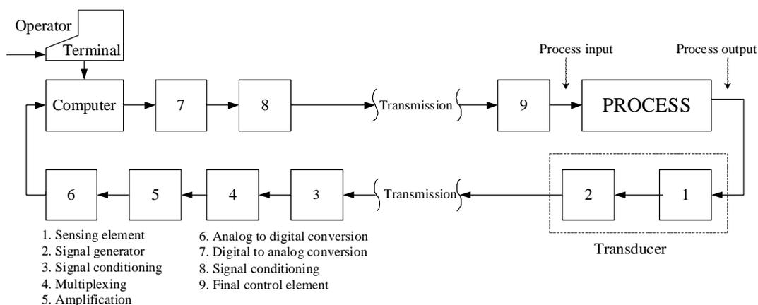
Figure 4: The component of a digital control loop
