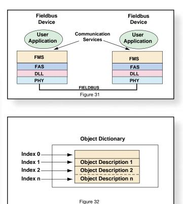
The object description is identified by its "index" in the OD. Index 0, called the object dictionary header, provides a description of the dictionary itself, and defines the first index for the object descriptions of the User Application. The User Application object descriptions can start at any index above 255.
