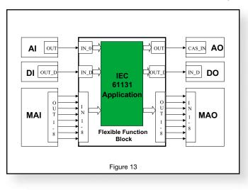
For example, a simple temperature transmitter may contain an AI function block. A control valve might contain a PID function block as well as the expected AO block. Thus, a complete control loop can be built using only a simple transmitter and a control valve (Figure 14).
