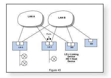
For example, a primary and secondary linking device are connected to the same H1 field-level network and the two redundant host-level networks providing two interfaces and two completely separate communication paths from the H1 fieldbus to the host. In case of any fault along the primary path, data can still pass through on the secondary path. This ensures that the plant floor data reaches the
